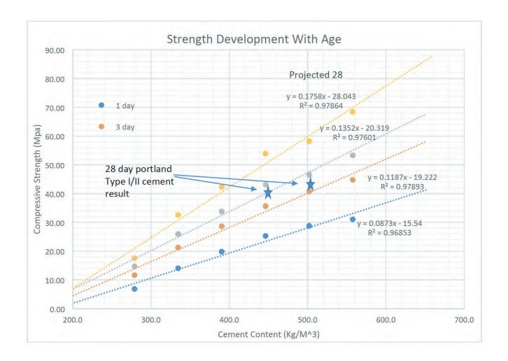
Benefits of utilizing sCMT is seen another way. In the case of what would normally be considered structural concrete the below table shows the relative strength difference between portland and sCMT mixtures. Options now exist to either yield higher strength concrete or the ability to reduce the binder content and cost per cubic meter.
